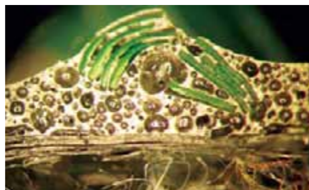
POLYURETHANE COATING To resolve this problem, Mondo has developed a special fixing process which involves the use of polyurethane coating.
