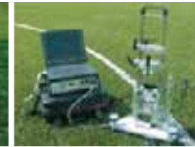
MEASURING SYSTEM FOR IMPACT FORCES AS PER DIN STANDARD 18035
