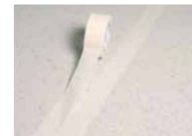
2 Protect the edges of the ground part with paper tape, leaving only the grinded track uncovered.
