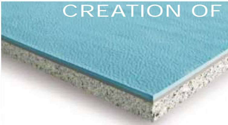
Mondo has introduced a modern composite made of three layers, the 1<sup>st</sup> and 2<sup>nd</sup> layers made of vulcanized rubber, a thermoset material and a 3<sup>rd</sup> layer made of a three-dimensional cross-linked polyurethane elastomer. The three layers combine during the curing/ manufacturing process to form the new generation MondoFlex gym surface.
