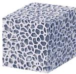
The open cell foam construction means that the foam bubbles (cells) remain mostly open, resulting after a critical stage in the foam-making process. This is a vitally important process to make a dense yet elastic polyurethane foam and create a three-dimensional cross-linked structure.
