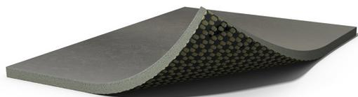
Everlay HIGH PROTECTION is a 7,5 mm thick stabilizing underlayment in rolls for sport flooring systems. It is composed of expanded PVC and reinforced with fiberglass, so it ensures enhanced stability, moisture resistance, high shock absorption and insulating properties. Its bottom layer is lightly textured with small embossed stems. It has been specifically designed to be loose laid over existing concrete subbase.
