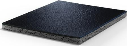
Prefabricated indoor sport flooring in rolls in a constant 10 mm thickness, consisting of natural and synthetic calendered and vulcanized rubber. Surface is hammered, opaque, non slip, anti-bacterial, marble-effect with uniform composition in 2 mm. This wear layer is vulcanized onto a load bearing, low hardness, low density, and flexible subfloor with a high content of recycled post-consumer material.
