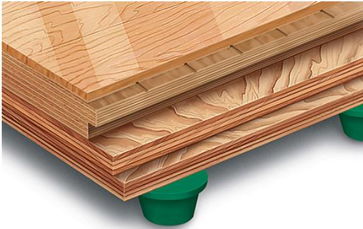
Areaelastic indoor flooring system, with a engineered hardwood (beech or oak) finish on top, built on site with several different layers in a total thickness of 62 mm:
