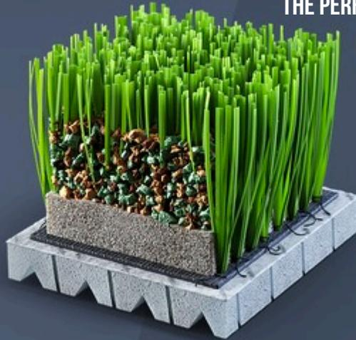
**DUAL PRO ANMX EF IS A NEXT-GENERATION ARTIFICIAL TURF SYSTEM COMPOSED OF 4NX MONOFILAMENTS WITH A SEMI-CONCAVE UPRIGHT STRUCTURE AND THREE ASYMMETRICAL RIBS, SATURN MONOFILAMENTS, WITH A STRAIGHT-STRUCTURE AND A CENTRAL SPINE, NATURAL MIX® TECHNICAL INFILL, AND PREFABRICATED ELASTIC UNDERLAYMENT IN RETICULATED POLYOLEFIN FOAM.**
