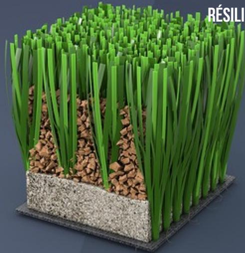
**SYSTÈME EN GAZON SYNTHÉTIQUE DE DERNIÈRE GÉNÉRATION COMPOSÉ D'UNE COMBINAISON DE MONOFILAMENTS 4NX À STRUCTURE DROITE SEMI-CONCAVE AVEC 3 NERVURES ASYMÉTRIQUES ET FILAMENTS FIBRILLÉS MONOFEEL, REMPLISSAGE DE PERFORMANCE EN LIÈGE CORK 120.**
