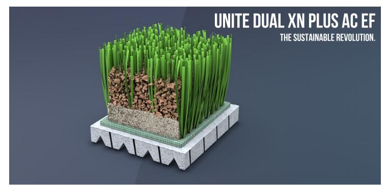
UNITE DUAL XN PLUS AC EF IS MONDO'S ARTIFICIAL TURF SYSTEM, COMPOSED OF AN INNOVATIVE COMBINATION OF XNOVA MONOFILAMENTS - WHICH FEATURE A STRAIGHT STRUCTURE AND PARALLELEPIPED SECTION WITH CONCAVE SIDES THAT FORM FOUR GROOVES AND 4 ASYMMETRICAL RIBS - AND 5NX MONOFILAMENTS, CHARACTERIZED BY A STRAIGHT STRUCTURE AND SEMI-CONCAVE SECTION WITH 3 ASYMMETRICAL RIBS, AND A THICKNESS OF 420 MICRONS.
