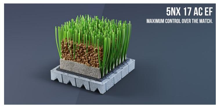
5NX 17 AC EF IS A NEXT-GENERATION ARTIFICIAL TURF SYSTEM COMPOSED OF 5NX MONOFILAMENTS WITH A SEMI-CONCAVE UPRIGHT STRUCTURE AND THREE ASYMMETRICAL RIBS, CORK 120 TECHNICAL INFILL, AND PRE-FABRICATED SHOCK-PAD IN RETICULATED POLYOLEFIN FOAM.
