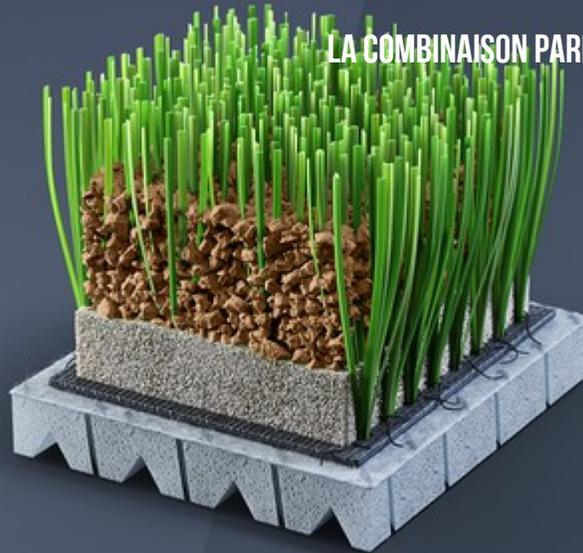
**SYSTÈME EN GAZON SYNTHÉTIQUE DE DERNIÈRE GÉNÉRATION COMPOSÉ DE MONOFILAMENTS 5NX À STRUCTURE DROITE SEMI-CONCAVE AVEC 3 NERVURES ASYMÉTRIQUES, REMPLISSAGE DE PERFORMANCE EN LIÈGE CORK 120 ET SOUS-COUCHE ÉLASTIQUE PRÉFABRIQUÉ EN MOUSSE DE POLYOLÉFINE RÉTICULÉE.**
