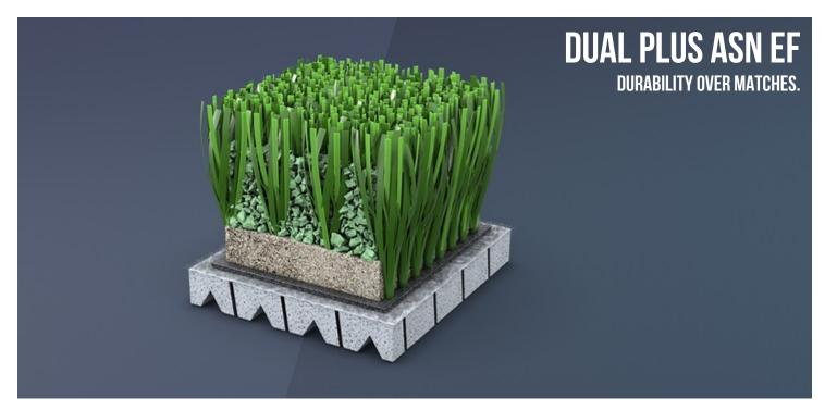
DUAL PLUS AER EF IS A NEXT-GENERATION ARTIFICIAL TURF SYSTEM COMPOSED OF 5NX MONOFILAMENTS WITH A SEMI-CONCAVE UPRIGHT STRUCTURE AND THREE ASYMMETRICAL RIBS, MONOFEEL FIBRILLATED FILAMENTS, ENCAPSULATED SBR GRANULES TECHNICAL INFILL, AND PREFABRICATED SHOCK-PAD IN RETICULATED POLYOLEFIN FOAM.
