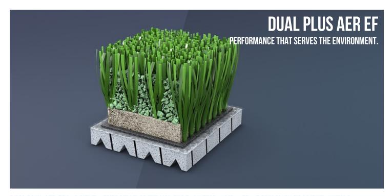
DUAL PLUS AER EF IS A NEXT-GENERATION ARTIFICIAL TURF SYSTEM COMPOSED OF 5NX MONOFILAMENTS WITH A SEMI-CONCAVE UPRIGHT STRUCTURE AND THREE ASYMMETRICAL RIBS, MONOFEEL FIBRILLATED FILAMENTS, ECOFILL® REBOUND TECHNICAL INFILL, AND PREFABRICATED SHOCK-PAD IN RETICULATED POLYOLEFIN FOAM.
