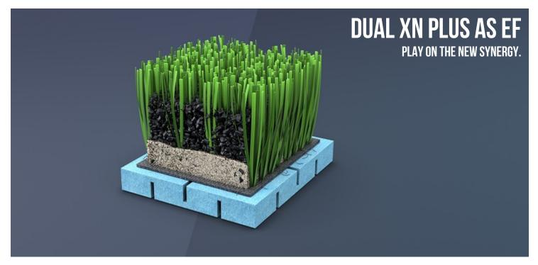
A STATE-OF-THE-ART ARTIFICIAL TURF SYSTEM THAT COMBINES MONDO'S NEW XNOVA MONOFILAMENTS WITH A Parallelogram-shaped structure with concave sides that form 4 grooves and 4 asymmetrical ribs, 5nx Monofilaments with a semi-concave structure with 3 asymmetrical ribs, performance infill made of SBR granules, and a prefabricated shock-pad in crosslinked polyolefin foam.
