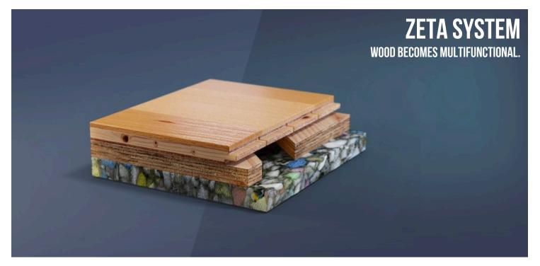
ZETA SYSTEM IS A FIBA LEVEL 1-CERTIFIED AREA-ELASTIC SPORTS SYSTEM CONSISTING OF A SINGLE LAYER OF PHENOLIC PLYWOOD CUT INTO FLOOR PANELS AFFIXED WITH A WOOD FLOORING AND FINISHED WITH A HIGH-RESISTANCE VARNISH. THE SYSTEM IS CUSHIONED BY A FLEXIBLE POLYURETHANE MAT, SUPPLIED IN TILES.
