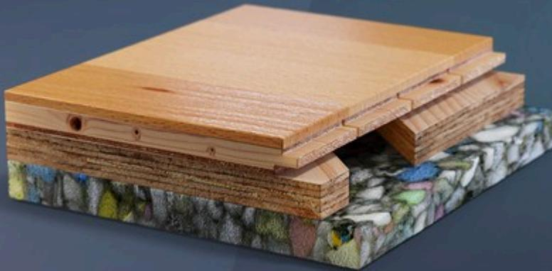
**ZETA SYSTEM EST UN SYSTÈME SPORTIF AREA-ELASTIC, HOMOLOGUÉ FIBA LEVEL 1, COMPOSÉ D'UNE SEULE COUCHE DE CONTREPLAQUÉ PHÉNOLIQUE DÉCOUPÉ EN LATTES, SUR LAQUELLE EST FIXÉ UN REVÊTEMENT PRÉFINI EN BOIS ET PRÉTRAITÉ AVEC UNE PEINTURE À HAUTE RÉSISTANCE. LE SYSTÈME EST AMORTI PAR UNE COUCHE DE SOUPLESSE FLEXIBLE EN POLYURÉTHANE EXPANSÉ, FOURNI EN DALLES.**
