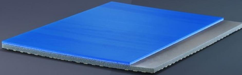
**THIS SYSTEM PAIRS MONDOFLEX RUBBER FLOORING WITH EVERLAY PROTECTION, AN UNDERLAYMENT WITH SUPERIOR STABILIZATION AND SHOCK ABSORPTION. IT CAN BE LAID LOOSE AND GUARANTEES SHOCK ABSORPTION VALUES OF BETWEEN 25% AND 34% (CATEGORY P1 ACCORDING TO STANDARD EN14904) TO ENSURE ATHLETES' COMFORT AND SAFETY.**
