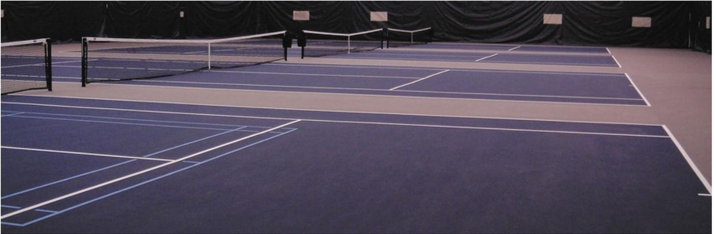
**MONDOTEN IS A UNIQUE, FACTORY-ENGINEERED, HIGH-PERFORMANCE SYSTEM WITH TWO PRIMARY COMPONENTS: AN ACRYLIC COATING SYSTEM AND A SHOCK ABSORPTION LAYER. COMBINED, THEY PROVIDE CONSISTENT AND TRUE BALL BOUNCE FOR THE LIFE OF THE SURFACE.**
