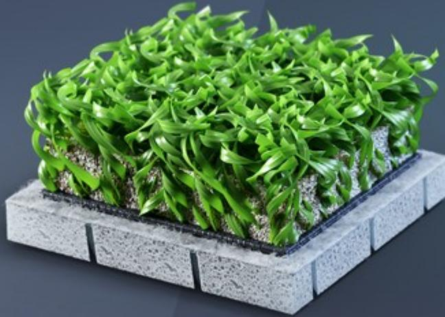
**MONDOHOCKEY GOAL IS A NEXT-GENERATION ARTIFICIAL TURF SYSTEM COMPOSED OF TEXTURIZED STX MONOFILAMENTS WITH AN UPRIGHT STRUCTURE AND TEXTURED CENTRAL SPINE, AND PREFABRICATED ELASTIC UNDERLAYMENT IN RETICULATED POLYOLEFIN FOAM.**
