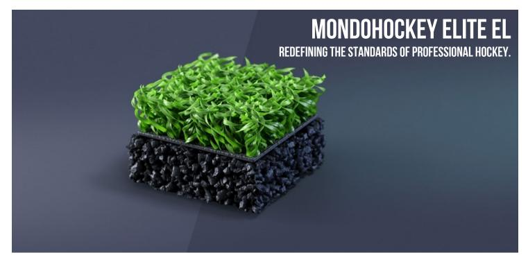
MONDOHOCKEY ELITE EL IS A NEXT-GENERATION ARTIFICIAL TURF SYSTEM COMPOSED OF TEXTURIZED 4NX MONOFILAMENTS WITH A SEMI-CONCAVE UPRIGHT STRUCTURE AND THREE TEXTURED ASYMMETRICAL RIBS, AND AN ELASTIC UNDERLAYMENT IN GRANULATED SBR CAST ON SITE. THE SYSTEM IS FREE OF INFILL AND MAY BE USED WATER BASED.
