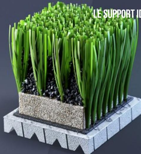
**SYSTÈME EN GAZON SYNTHÉTIQUE DE DERNIÈRE GÉNÉRATION COMPOSÉ D'UNE COMBINAISON DE MONOFILAMENTS 4NX À STRUCTURE DROITE SEMI-CONCAVE AVEC 3 NERVURES ASYMÉTRIQUES ET FILAMENTS FIBRILLÉS MONOFEEL, REMPLISSAGE DE PERFORMANCE EN SBR OU SBR ENNOBLI ET DESSOUS DE TAPIS ÉLASTIQUE PRÉFABRIQUÉ EN MOUSSE DE POLYOLÉFINE RÉTICULÉE.**
