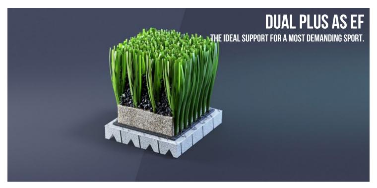
DUAL PLUS AS EF IS A NEXT-GENERATION ARTIFICIAL TURF SYSTEM COMPOSED OF 5NX MONOFILAMENTS WITH A SEMI-CONCAVE UPRIGHT STRUCTURE AND THREE ASYMMETRICAL RIBS AND MONOFEEL FIBRILLATED FILAMENTS, TECHNICAL INFILL IN SBR OR ENCAPSULATED SBR, AND A PRE-FABRICATED SHOCK-PAD MADE FROM RETICULATED POLYOLEFIN FOAM.
