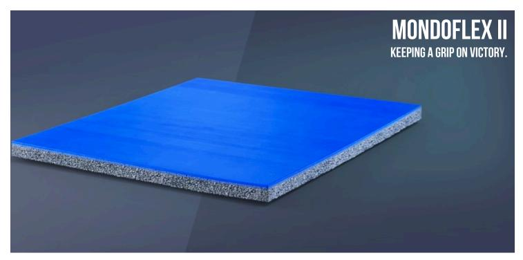
MONDOFLEX II IS A POINT-ELASTIC SPORTS FLOORING WITH SHOCK ABSORPTION VALUES ABOVE 25% (CATEGORY P1 ACCORDING TO REGULATION EN 14904). THE FLOORING COMPRISES TWO LAYERS OF NATURAL AND SYNTHETIC RUBBER THAT ARE JOINED IN THE PRODUCTION PHASE TO A SUPPORTING UNDERLAYMENT OF ELASTIC FOAM. PRE-FABRICATION GUARANTEES THAT THE PRODUCT IS UNIFORM WHEN INSTALLED AND ENSURES A CONSTANT BIOMECHANICAL RESPONSE ACROSS THE ENTIRE SURFACE.
